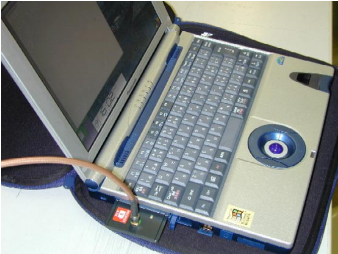
This LAN card has a SMA connector for antenna cable
