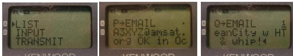
Figure 1. This shows the message menu and a typical APRS message. In this case, instead of a message to a callsign, it is a message to EMAIL which causes the APRS system to convert it to standard email for ultimate delivery. The actual email address is included as the first word in the message such as [A3XYZ@AMSAT.ORG](mailto:A3XYZ@AMSAT.ORG) as shown here. The text is “OK in OceanCity w HT & whip!” which I was using for a satellite test.
