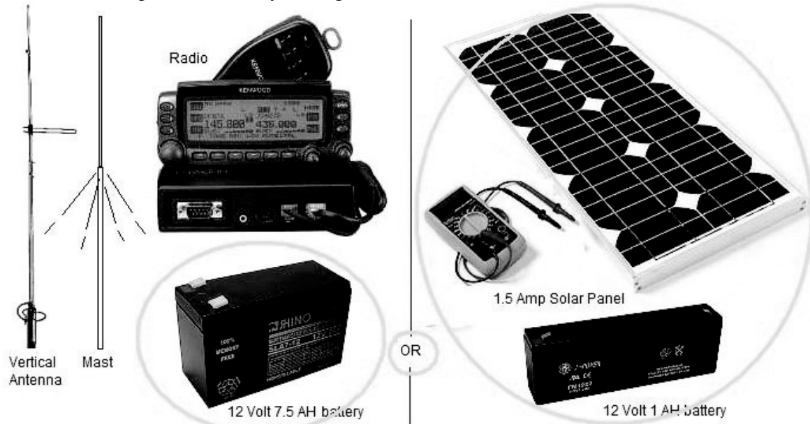
Figure 5. Typically about 1.5 Amp Hours per hour is the average power drawn for such a portable digipeater. Figuring out the long term power for such an ad-hoc station is part of the challenge. Several other creative power techniques were used at the 2009 event[4].
