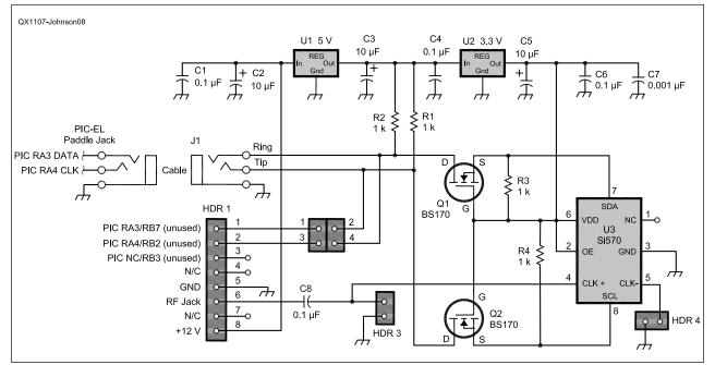
Figure 8 — The Si570 daughtercard schematic diagram.
