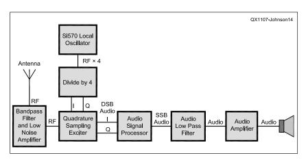
Figure 14 — This block diagram represents a CW or SSB Receiver.
