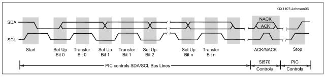
Figure 6 — The IC2 data transfer timing diagram.
