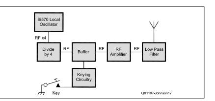
Figure 17 — A 40 m CW Transmitter is shown in this block diagram.
