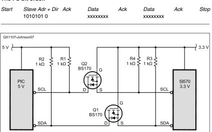
Figure 7 — This circuit shows an I<sup>2</sup>C level shifter.
