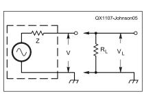
Figure 5 — A basic test circuit to measure the Si570 output impedance.
