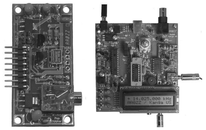
Figure 10 — Here, the Si570 daughtercard is plugged into the PIC-EL III board.
