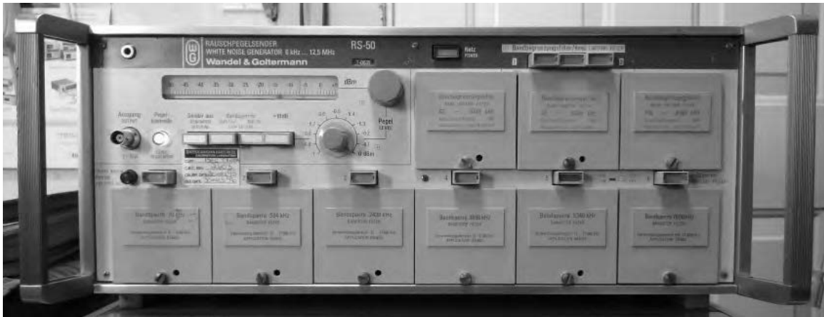
Fig.6: The Wandel & Goltermann RS-50 White Noise Generator.
