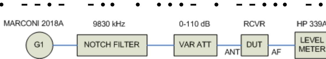
BLOCK DIAGRAM OF RECIPROCAL MIXING TEST SETUP
