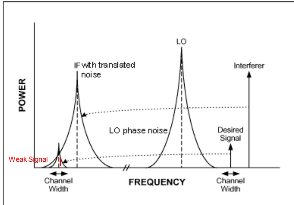
Strong interferer mixes with LO phase noise to “throw” noise into IF channel. If the interferer consists of wideband noise, the IF channel will be filled with noise.
