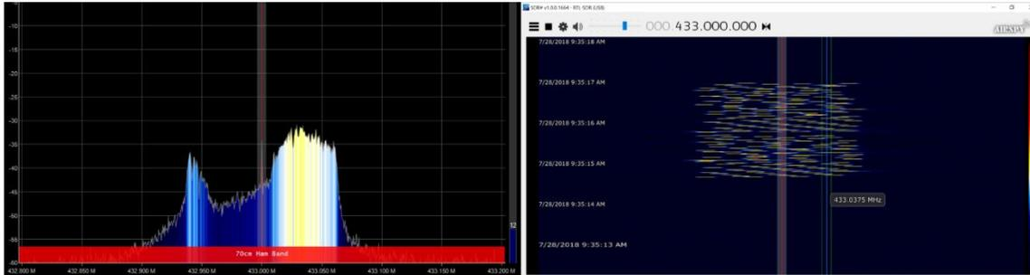
Figure 2: Spectrum analyzer view of the LoRa spread spectrum waveform. Left hand image shows the 125KHz bandwidth of the 300bps LoRa setting, while the righthand image shows a waterfall diagram of the LoRa transmission. While the righthand image partially shows the chirp modulation, the limited sample rate of the RTL-SDR (maximum 3.2Mps) provides a waterfall with a limited resolution, even with the FFT set to the minimum of 512 samples.
