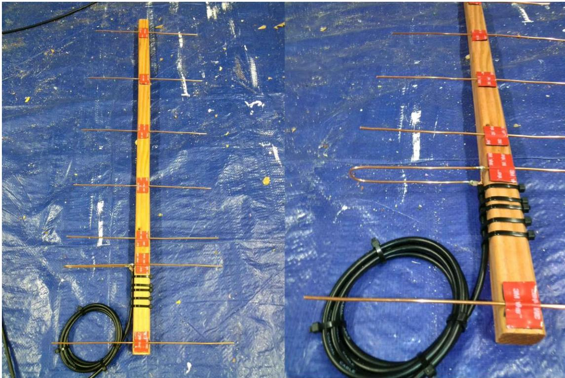
*Figure 6: Portable Yagi antenna used for dismantled mobile experiments.*
