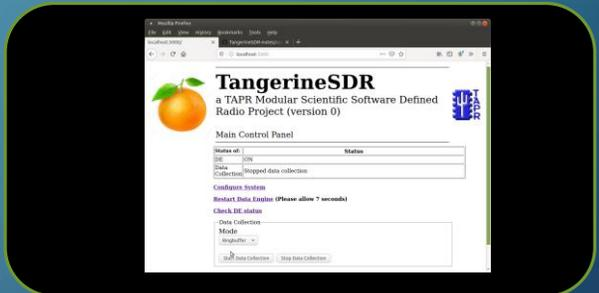
Local Browser-based UI “Web Controller” (running flask, flask-WTForms)
