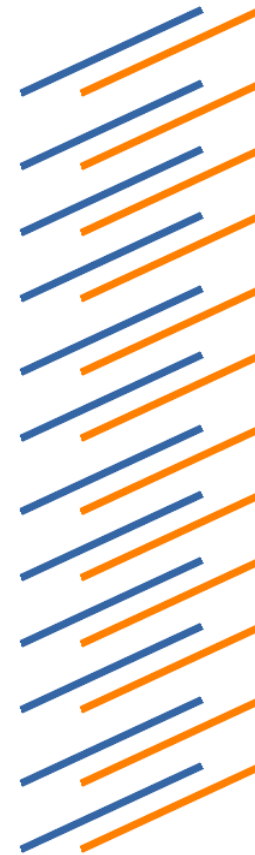
Two LoRa signals with a small frequency offset
