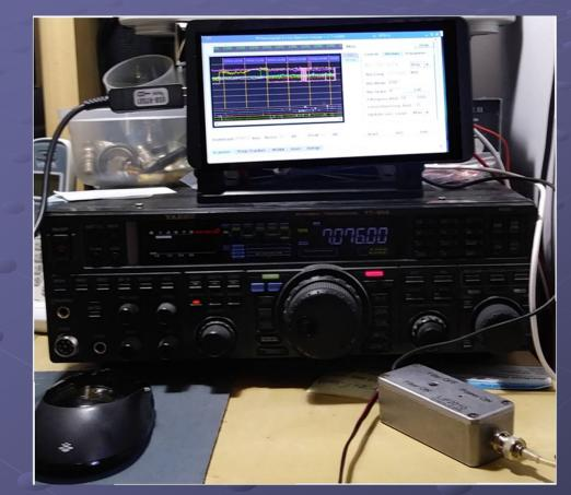
5V 2A power is supplied via a 12V car power adaptor. The LIF interface (cast metal box) requires 12V/10mA power.
