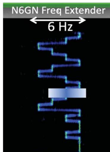
Figure 3. Waterfall display of the spectrum of the 33rd harmonic of a 14 MHz local FST4W-120 transmission from on ANAN SDR at N6GN using a KīwiSDR with GPSDO and a homebrew frequency extender. The image shows the smooth transitions between tones and the fraction of a tone period they span. The rectangle at the centre represents additional spectral spreading.
