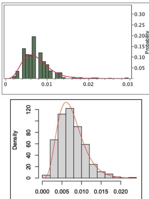
Figure A1. (upper) Histogram of actual spectral width values in Hz over a 21 km line-of-sight path from N6GN to N6GN/K with identical GPDSO master oscillators at the transmitter and receiver with a best-fit Gamma distribution. (lower) A synthesised histogram of a Gamma distribution of 500 values with the same Scale and Shape parameters as the observations.
