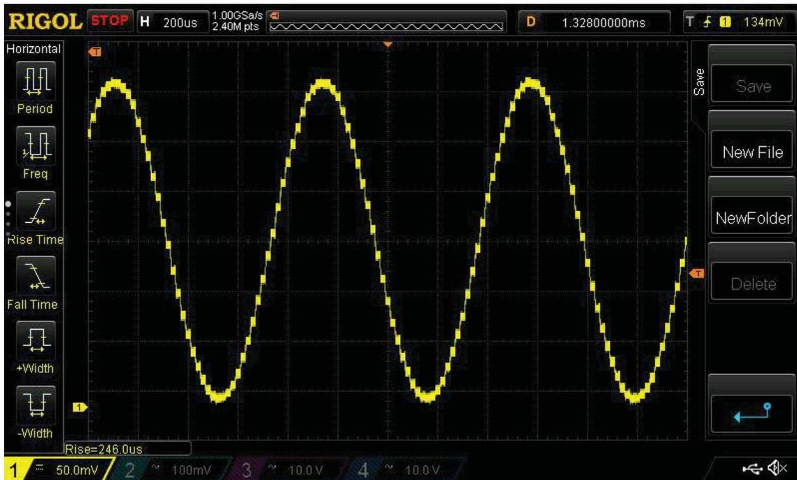
This is a comparison scope view of the raw output from the DAC, output of the op-amp section and just past the low-pass filter before going through the 10K transmit level potentiometer.
