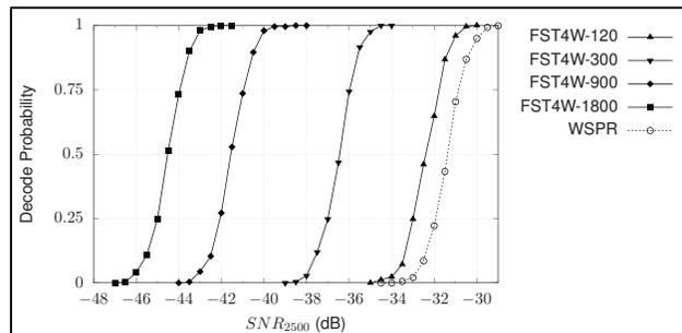
Figure 2. How decode probability varies with SNR near the threshold for FST4W-120 to -1800 in comparison with WSPR. Acknowledgement: figure provided by Steve Franke K9AN.
