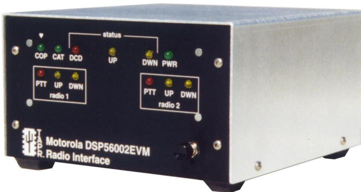
The DSP56002EVM comes with Motorola's DSP56000 cross-linker Assembler and Domain Technologies' debug software with windowed user interface. The software runs under MS-DOS on an IBM PC-compatible computer (386 class or higher) and communicates with the evaluation module over an RS-232 serial port.
