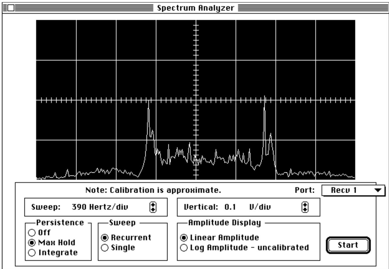
*Spectrum Analyzer: The display shows a 1200 bps packet audio signal. Note the two peaks corresponding to the low and high tones of the AFSK signal.*
