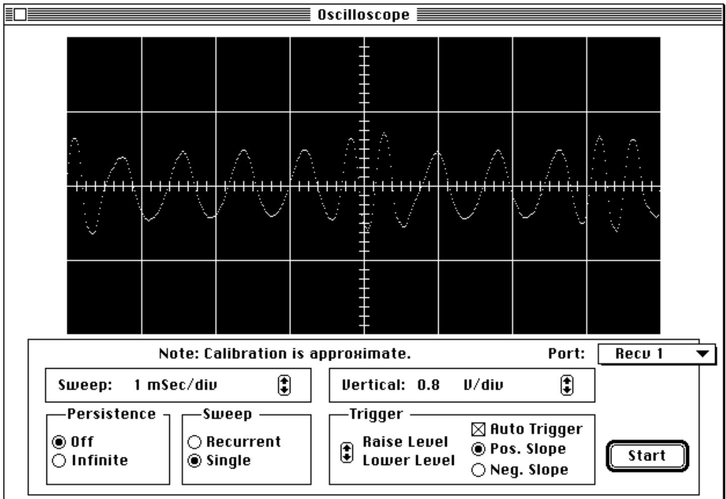
*Oscilloscope: The display shows a 1200 bps packet audio signal. Note the two different periods of the waveform corresponding to different binary digits.*
