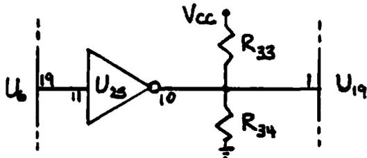
Figure 1. Revised CWID facility for the TAPR TNC.
