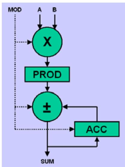
FIGURE 21 – MULTIPLY-ACCUMULATE UNIT
