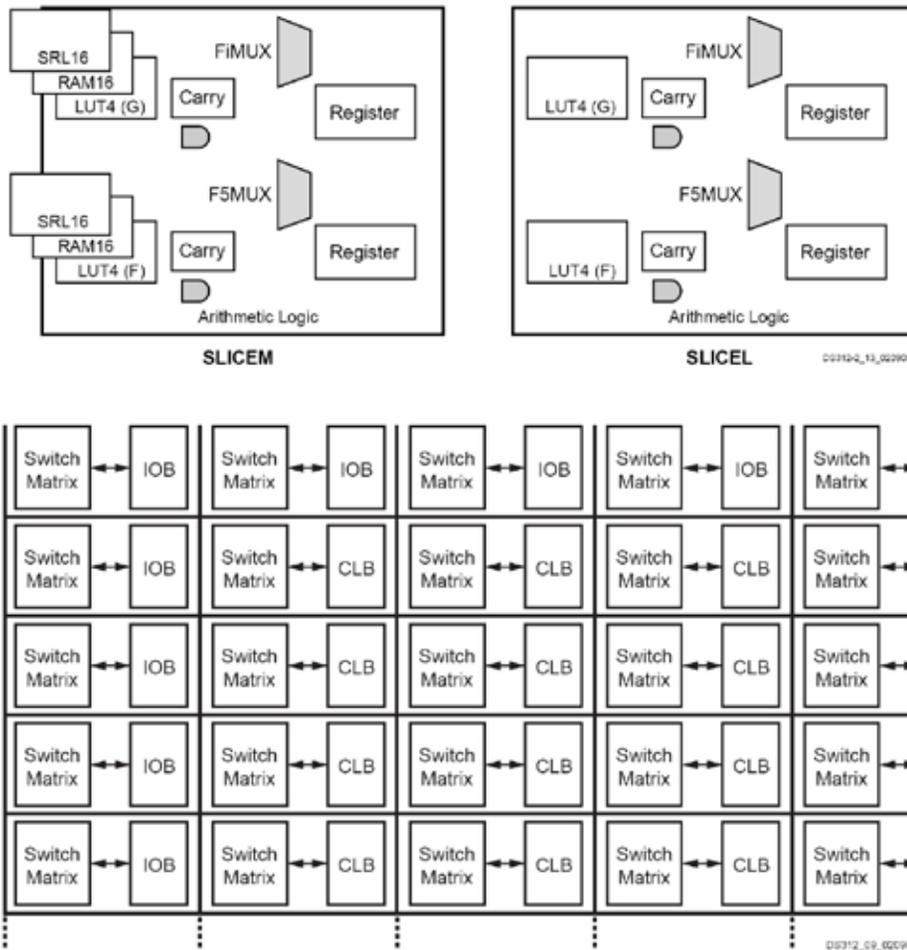
FIGURE 1 – FPGA ARCHITECTURE
