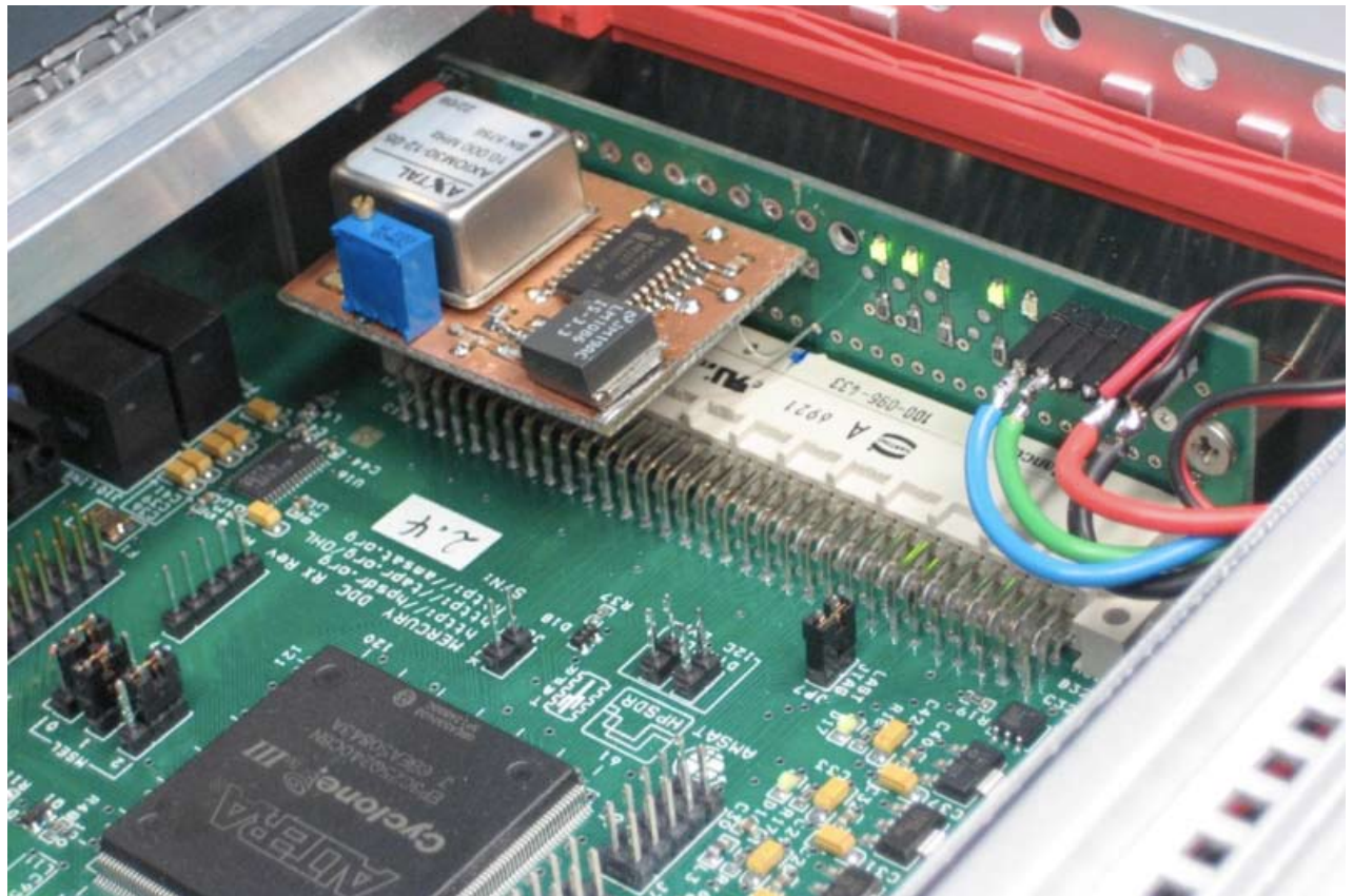
Fig.11: The photo shows the Axtal 10 MHz OCXO mounted on a small printed circuit board connected to the Atlas board of the hpSDR transceiver (9). It is used as the clock source in this fully digital transceiver system and determines its frequency accuracy and stability.
