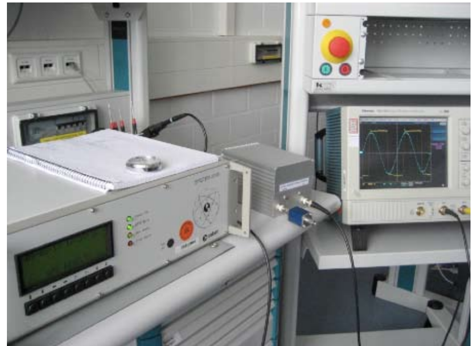
Fig.8: Test set-up comparing the 10 MHz signal from a GPS locked Rb-standard (left) with the signal delivered by the surplus unit described before (centre). Both signals are applied to an oscilloscope to compare frequencies by measuring their beat period.
