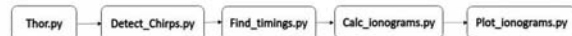
Figure 3. The steps involved in data collection and execution of the Chirpsounder2 software package.
