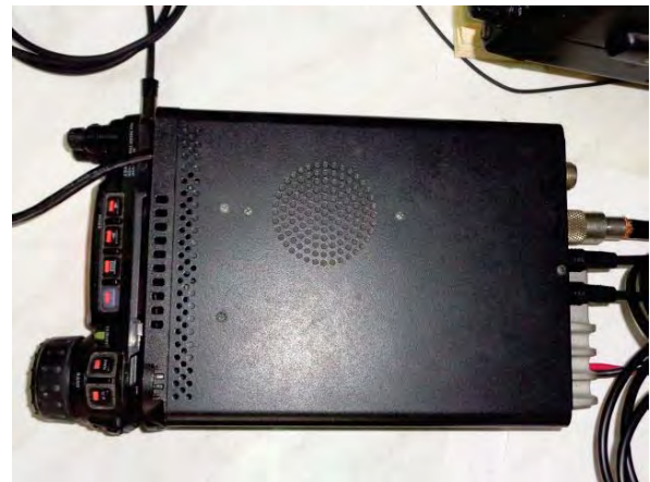
Figure 7. Two cables on the backside (pactor), and two cables on the front (packet).
