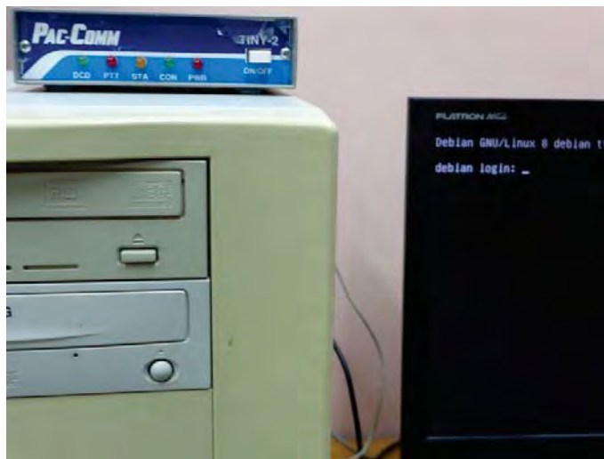
Figure 2. Pac-Comm terminal node controller planned for the BBS operation.
