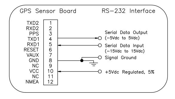
connector attached directly to the sensor board (+5V @ 15 mA power is supplied on the center conductor for the antenna).
