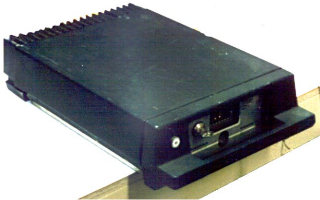
MOCOM 70 — 25 Watt version. Note the size of the heat sink as compared to the 50/75Watt below. The 25W version has heatsink fins, while the 50/75W does not.
