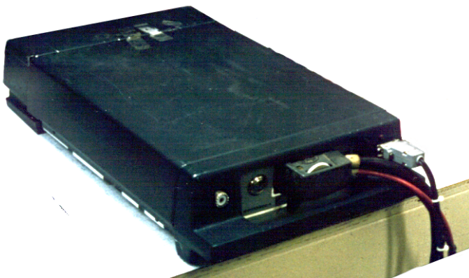
MOCOM 70 — 50/75 Watt version. Note the different style and size of the PA section on the rear. This picture also shows the control head and radio connection (DB9).
