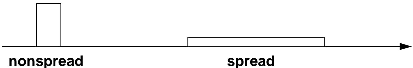
**Spectral density (W/Hz) x Bandwidth = Total power
