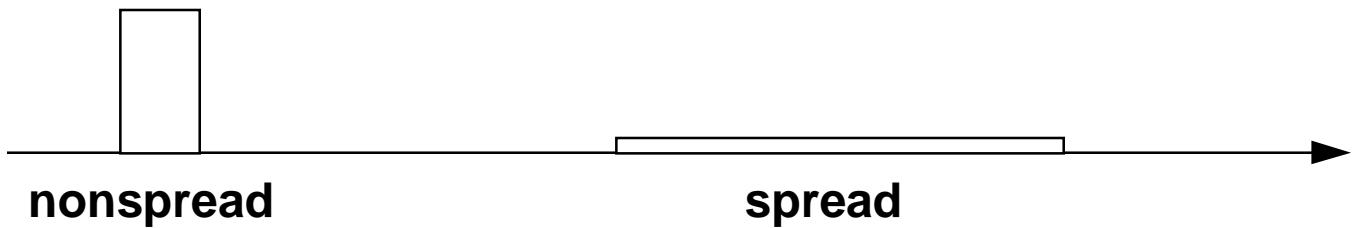
area of spread signal now less than nonspread signal
