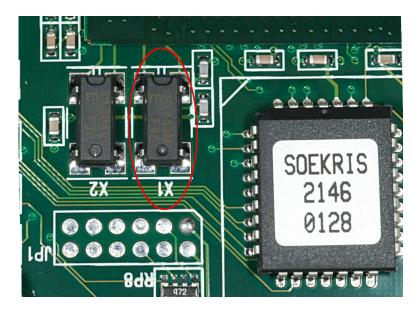
Next, remove X1. A small heat gun is the best way to heat all four pads simultaneously, though with care a soldering iron and solder wick can do the job. If you happen to lift any of the pads, you have three chances out of four that won't be a problem – we'll only be using one pad, the one at the upper left (when looking from the front of the board).
