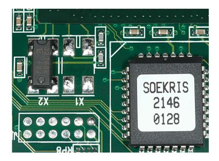
The net4501 CPU uses 2.5 volt logic, so the signal from the Clock-Block, even when using the 3.3 volt regulator, is a little high. A 100 ohm resistor between the clock input and ground will reduce the signal to an appropriate level. The resistor is positioned with one lead on the upper left pad of X1, and the other soldered to the upper right pin of JP3. A piece of RG-174 coax is soldered across the resistor, with the center conductor going to X1, and the braid to the ground at JP3:
