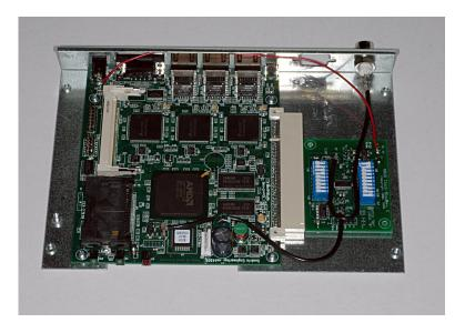
The Clock-Block needs to generate 33.333333 MHz, so set the jumpers according to the table above.
