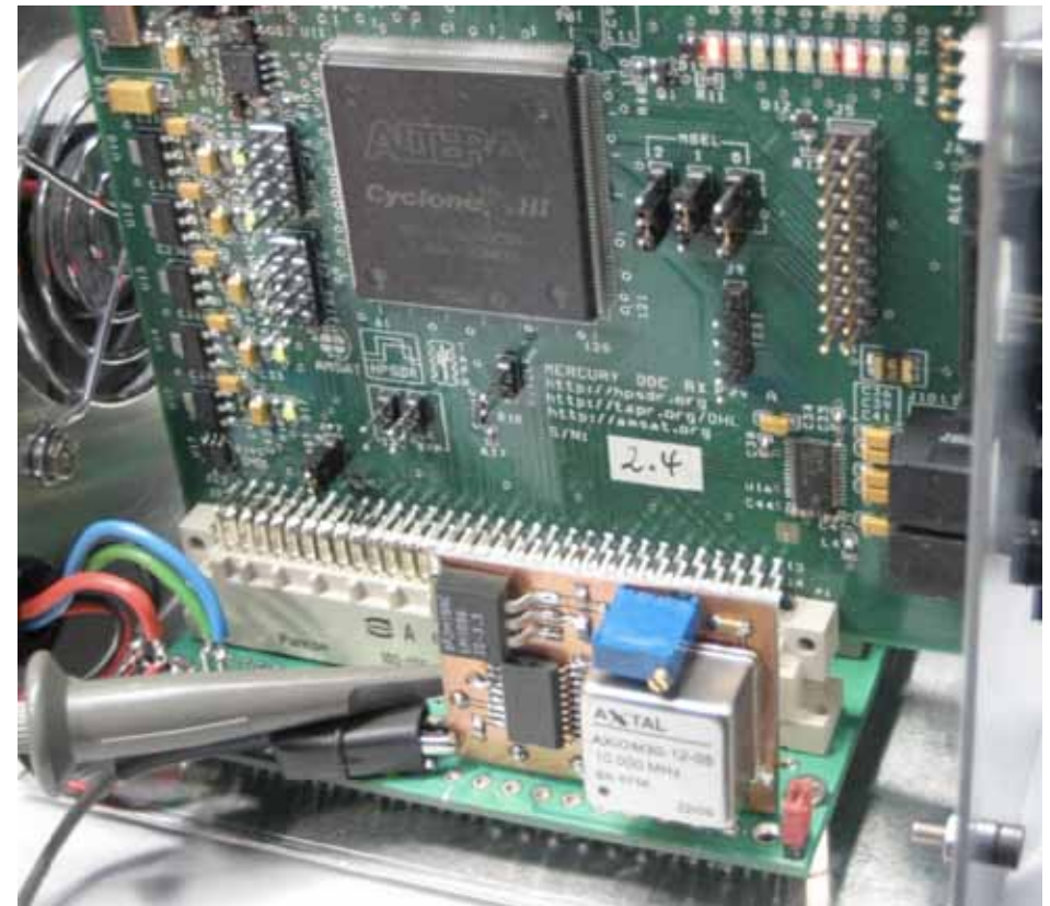
Figure 7. The clock board on Atlas and all other boards assembled (MERCURY in the background) during clock pulse measurements with the probe tips connected to the output.
