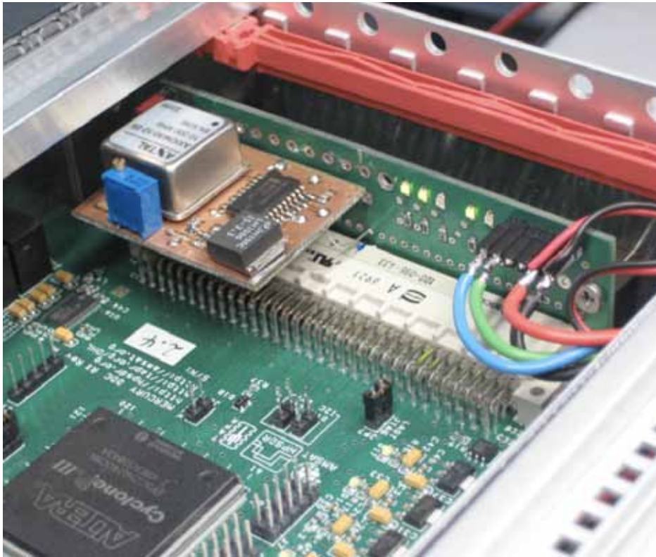
Figure 8. All boards installed into the hpSDR cabinet which contains in addition the linear regulated necessary power supplies (+12V, -12V, +5V) and a 10W class-A driver amplifier following Penelope. Connection to C16 of Atlas is done with the non-isolated wire at the lower right of the small print board.
