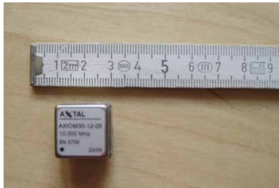
Figure 1. The oven controlled low phase noise 10 MHz quartz oscillator model AXIOM30-12-05 by AXTAL. Current consumption is 180 mA during warm up, 60 mA in steady state phase. Output is 5Vpp HCMOS.
