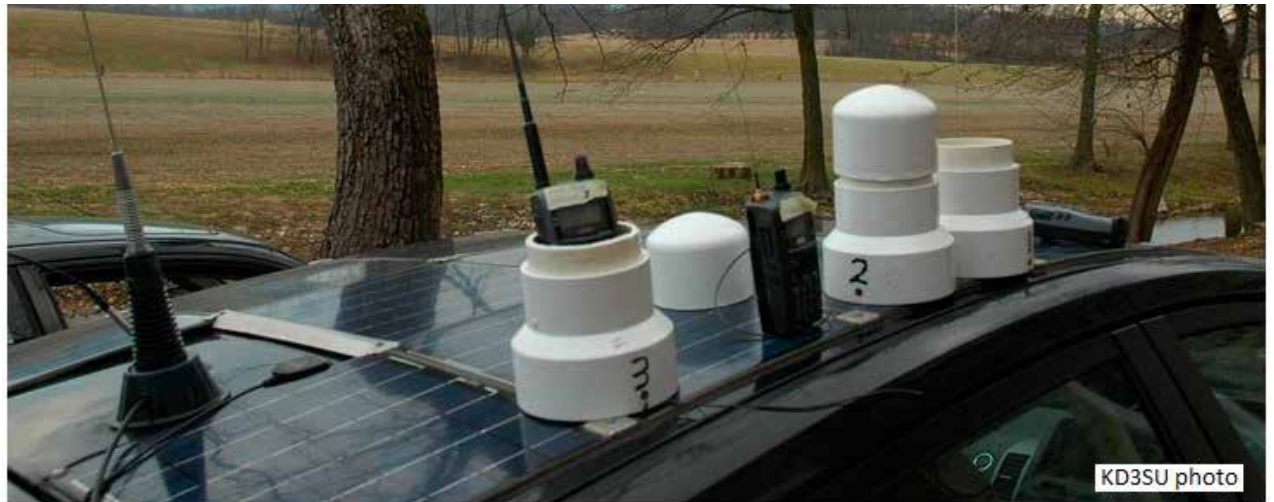
Fig. 2: Three of the cave digipeaters (with or without tops). The HTs just drop in and out for easy adjustment.
